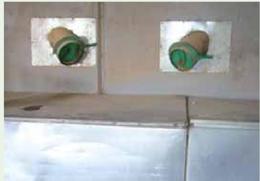
Feed is drawn on from the hopper bins as required eliminating the need to manually handle large, bulky and awkward bags.
